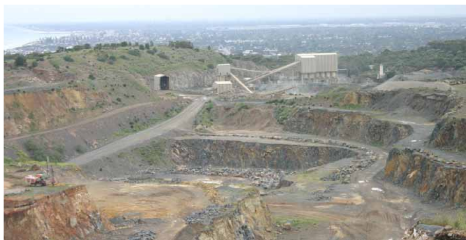
Figure 3 Linwood Quarry showing the view north to crushing plant and Adelaide city area. The quarry is located ~15 km SW of Adelaide CBD and produces limestone for aggregates, road base and rail ballast. (Photo 408319)
